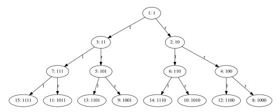
The nodes in this tree are annotated with the both the decimal and the binary representation of their keys. The root node is for key 1; key 0 is not allowed. All values in the right subtree are even, while all values in the left subtree are odd. This means that the last digit is always 0 or always 1 depending on the subtree. We then continue with this scheme recursively. At level 2, we look at the second bit, level 3 looks at the third bit, and so on.
